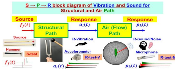
Figure 1: Source-Path-Response (SPR) system block diagram [7].
