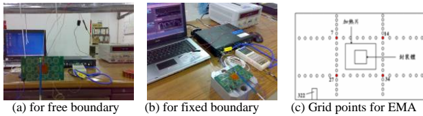
FIGURE 2. EXPERIMENTAL SETUP FOR EMA OF PCB
