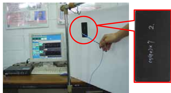
Figure3 Experimental setup for carbon plate EMA
