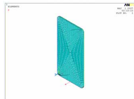
Figure 4 FE model for carbon plate
