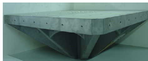
Figure 2: 750 type auxiliary table of vibration testing machine
