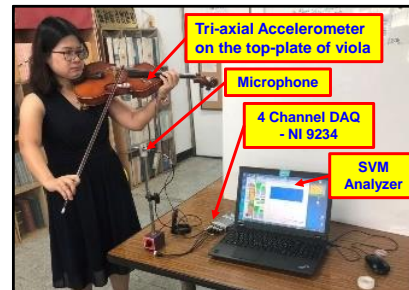
Figure 3: Experimental setup for sound and vibration measurement.
