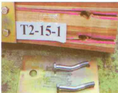
Fig. 5. Shear failure occurring along each row of bolt holes parallel to the grain of a glulam member.
