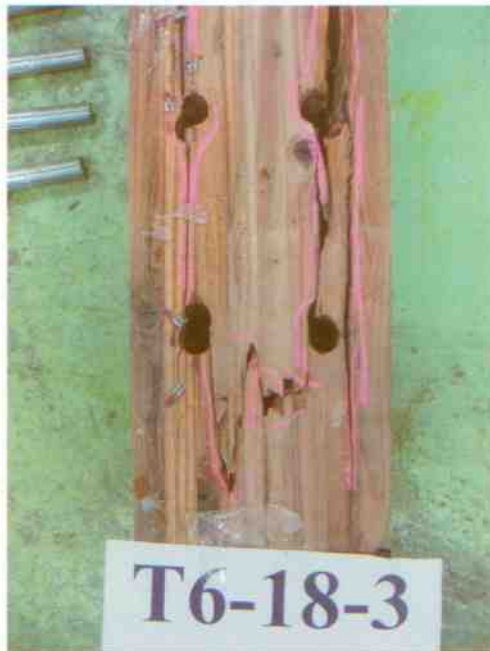
Fig. 13. Resultant Y-shaped split of a glulam member at failure during the tensile test.
