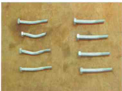
Fig. 8. Yield failure of bolts. (left: 15-mm bolts; right: 18-mm bolts).
