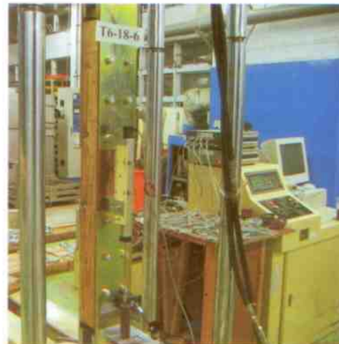
Fig. 2. Configuration of the bolt joint tensile test apparatus with steel plates for structural glulam members.
