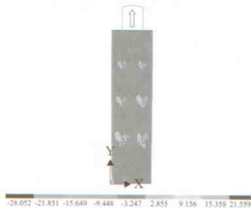
Fig. 12. Simulated shear stress ( \tau_{xy} ) distribution of a glulam member subjected to 10% of the maximum tensile load at failure (3250.8 kgf).
