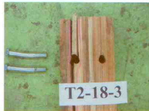
Fig. 6. Shear failure pushing a woodblock from the bolt holes to the end of a glulam member under tensile loads.
