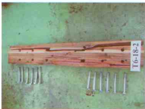
Fig. 7. Overall split along a glulam member connected with 18-mm bolts.
